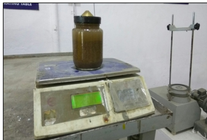
Figure 3.2 Specific gravity test of fine sand using pycnometer
