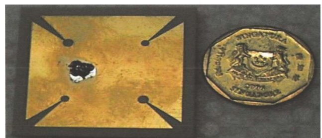
FIGURE 3: Compact antenna with symmetrical slit [46]. an impedance bandwidth of 3.8 GHz, operating from 4.2 to 8 GHz [42]. In comparison, a wider impedance
